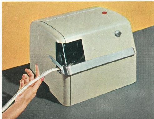
Teletype Model 28 Tape Punch. Receives incoming electrical signals, punches a 5-level "common language" tape, and prints the data right on the tape, for easy identification and handling. This unit is used for message relaying . . . for integrating data from several sources into a single tape . . . and for providing punched tape as a by-product of send-receive operations.
