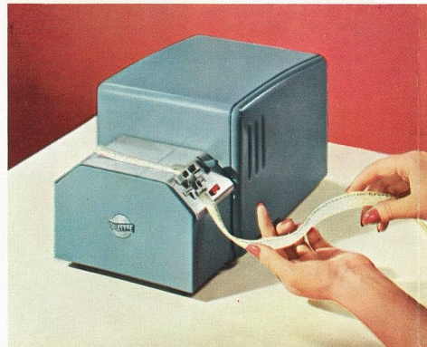
Teletype Model 28 Tape Reader. This is a sending unit. Reads punched tape and instantaneously transmits data to local or remote receiving equipment. As with all Teletype transmitting units, data may go to one destination or a number of destinations simultaneously—either nearby or thousands of miles away.
