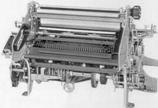
Rear view of Teletype Model 28 typing unit with area occupied by stunt box shown in red.
