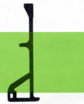
154639 Slide — Used for operating shift fork by one to four, adjacent function levers
